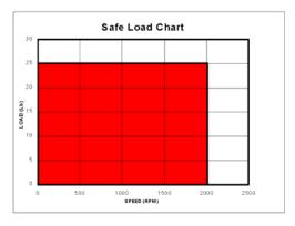
The area below 25 pounds and less than 2000RPM is the recommended load region.
