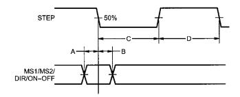
For the sinking version (23MDX06X-XX-00-XX) the inputs are considered inactive or Logic "1" if left open, or active or Logic "0" if grounded. For the sourcing version (23MDX06X-XX-24-XX) the inputs are considered inactive or Logic "0" if left open, or active or Logic "1" if pulled to 3.5 - 24VDC.
